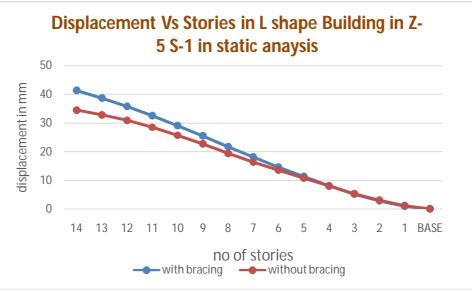
Graph: 2 Displacement variation along zone 5 soil-1 in static analysis
