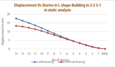
Graph: 1 Displacement variation along zone 2 soil-1 in static analysis
