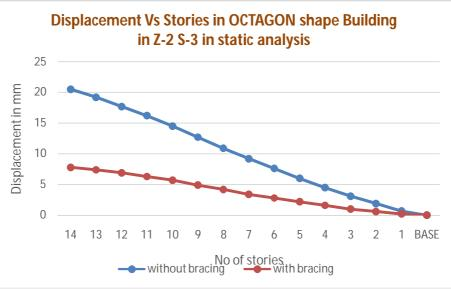
Graph: 7 Displacement variation along zone 2 soil-3 in static analysis
