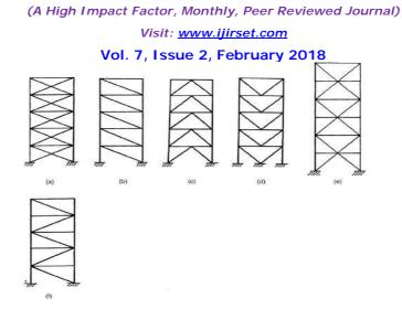
Figure 1 Typical concentric braced frame (CBF) configurations: (a) One-storey Xbracing; (b) Single-diagonal bracing; (c) and (d) Chevron bracings; (e) two-storey Xbracings; (f) Single-diagonal alternate-direction bracing.
