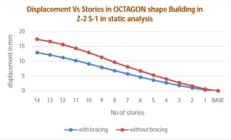
Graph : 5 Displacement variation along zone 2 soil-1 in static analysis
