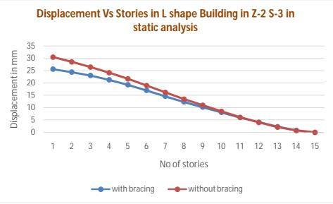
Graph: 3 Displacement variation along zone 2 soil-3 in static analysis
