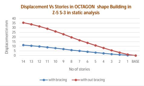
Graph: 8 Displacement variation along zone 5 soil-3 in static analysis.
