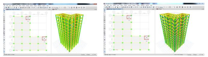
Figure:1 Model showing of L-Shape with and without steel bracings
