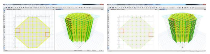
Figure:2 Model showing of Octagon-Shape with and without steel bracings
