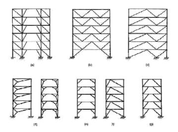
Figure 2 : Brace configuration that allows for door-size openings in interior space layouts.
